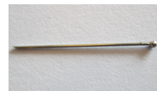
FIGURE 2.7: Single point scatterer used in experiments
