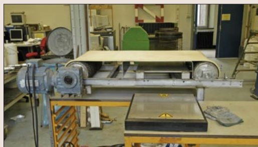
The 2 litre blob is held in place by a heavy permanent magnet located directly below the belt. The magnet consists of nine poles and weighs about 120 kilograms.
