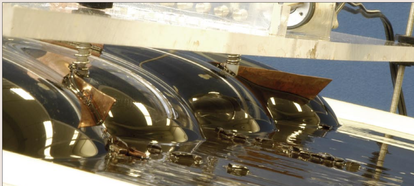
A separator vane inserted into the fluid down to 2 cm above the belt is used to separate the floating particles from those lying on the belt. The heavier particles move under the vane and drop off the end of the belt. The lighter particles float over the vane to hit a V-shaped ridge that carries them away to the side of the belt.
