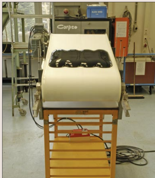
Test set-up of an inclined conveyor belt carrying a large blob of magnetic fluid, used for separating different types of metal.
