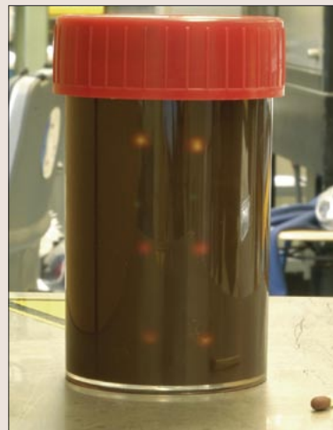
If a lump of magnesium (density approx. 1700 \text{ kg/m}^3 ) is dropped into a manganese chloride solution (density approx. 1400 \text{ kg/m}^3 ), it sinks to the bottom. If the container holding the solution and the metal is then placed on a magnet, the metal will rise in the solution (picture on the right) because of the increased density of the fluid.
