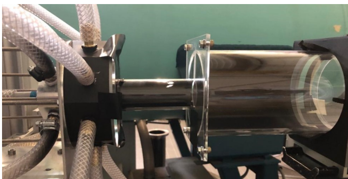
Figure 5.13: Centre-plane setup with reflection reduction
