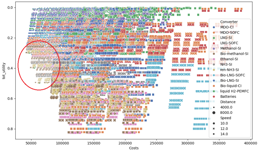
Figure 3.7: Total utility versus cost for different options over multiple epochs, with varying design speed and sailing distance. The total utility has been reversed to ensure the preferred options are in the bottom left.
