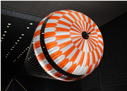
(a) The 70.5 ft diameter parachute that delivered NASA's Perseverance Rover to the Martian surface [Airborne Systems, 2020]
