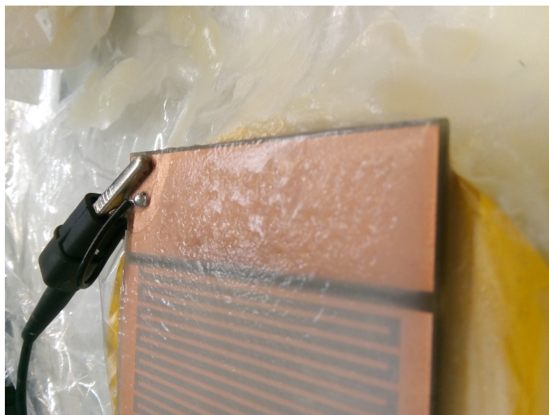
Figure A-2: The thickness measurements with the Elcometer change the surface.
