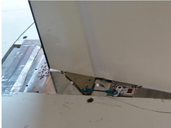
*Figure 3.8: Trailing edge flap and servo motor on the DU 95-W-180 experimental model.*
