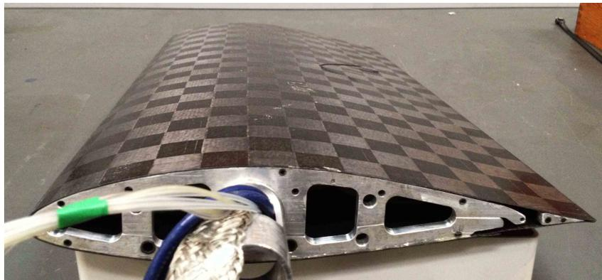
*Figure 3.3: Closed wing as used during measurements.*
