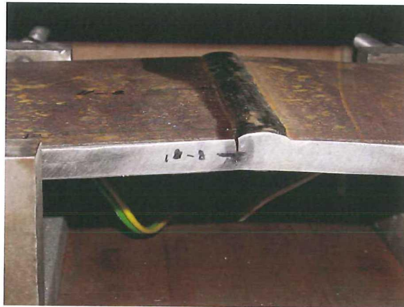
Figure 7. Typical fatigue crack at the weld toe
