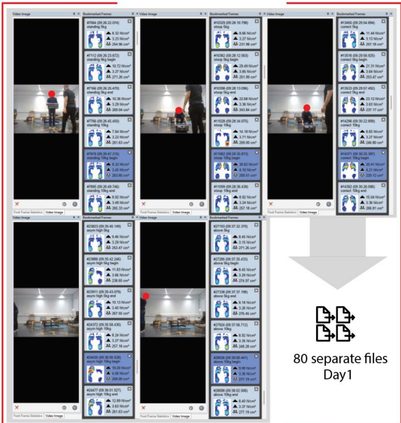
Figure 18: every posture is labeled manually with a begin and end bookmark in the xsensor software.
