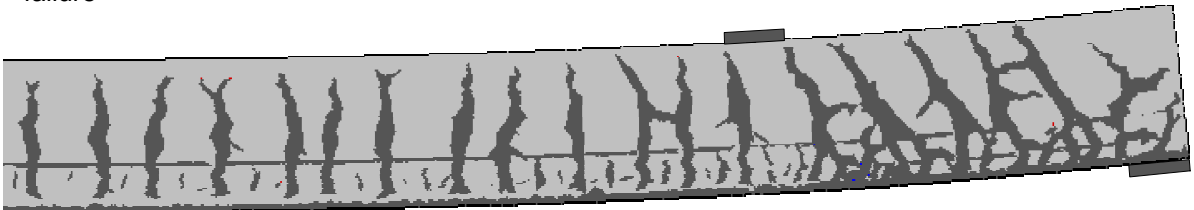
Figure 7.11: Comparison between calculated and measured crack pattern in R-HVP260S-11 specimen.
