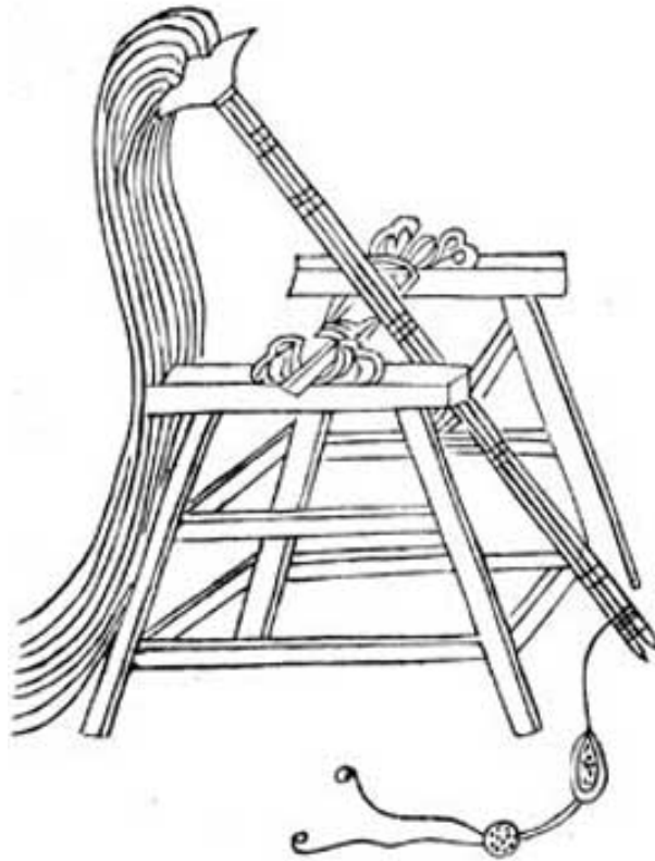
Figure 1.1: A drawing of an original mangonel where the beam would be pulled down by soldiers rather than by a counterweight. The projectile would be put in the sling which is depicted in the bottom right. The updated mangonel which had a fixed counterweight would have had the counterweight where the pulling ropes are now attached. [2]
