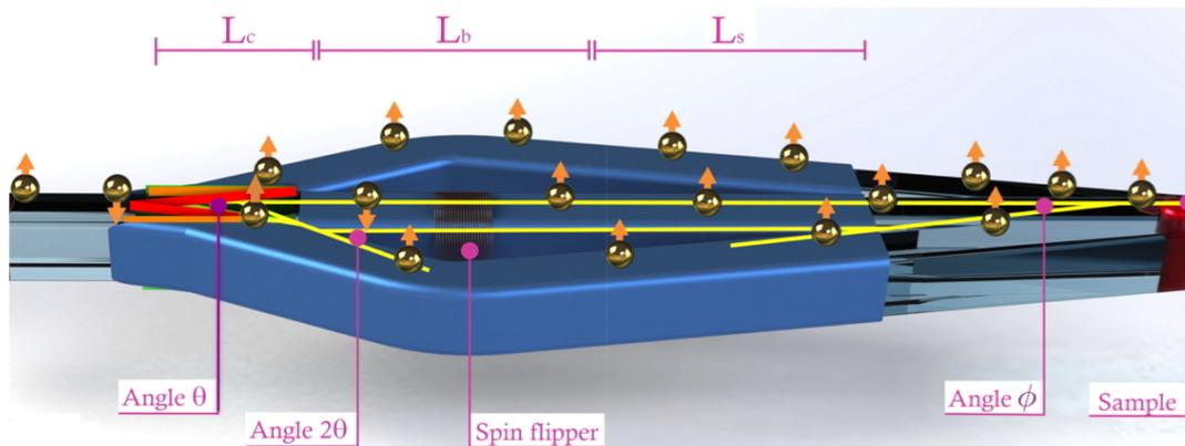
Figure 3: Artist's view of the setup of fig. 2 illustrating the geometry and an RF flipper positioned at the central beam. The drawing is not in scale.
