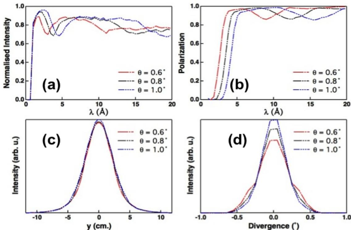
Figure 5: Normalised neutron intensity (a), polarisation (b), horizontal beam profile (c) and divergence (d) of the system for three values of the angle  $\theta$  for the polarising cavity. The simulations correspond to the case “1 LOS” assuming the characteristic lengths given in Table 2.
