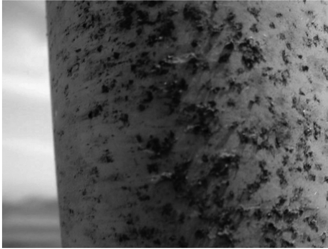
FIGURE 4.6 Contamination by insect debris on the leading edge of a wind turbine blade in Magallón 26 wind farm in Zaragoza, Spain ( Blade cleaning.com ).
