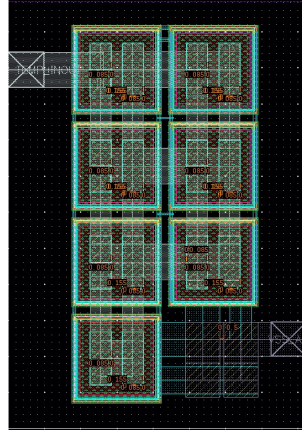
Figure 4.16: Layout of the BJT temperature sensor
