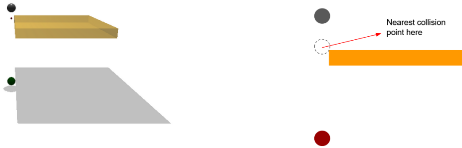
Figure 4.3: Collision point along a trajectory found in Chai3d. Unlike the collision points found by traditional physics engines, Chai3d finds the exact position where the center of the proxy will end up on a given trajectory.
