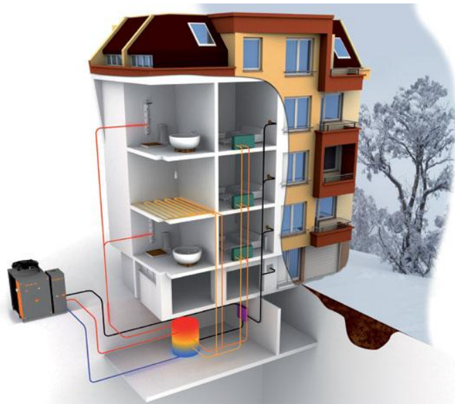
Figure 20. Air source gas absorption heat pump used for hot water and space heating. 3
