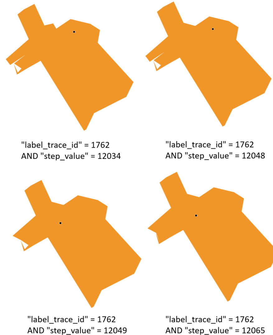
Figure. Anchor displacement due to geometry change in one face
