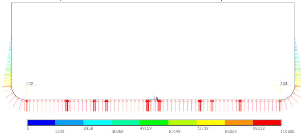
Figure 20 – Hydrostatic pressure midsection [Pa]
