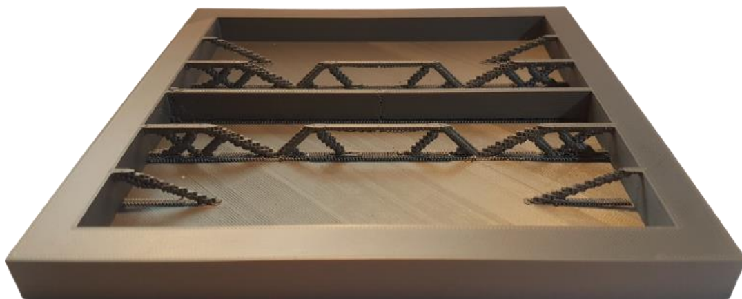
Figure 8 – 3D print result of the simply stiffened plate for the case of 4 templates per type (Bakker, 2020)
