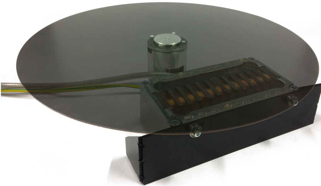
Figure 3.16: Dynamic setup, the rotor made transparent as to show placement of underlying components. The rotor can be seen to be supported in the middle by the bearing mount that also contains the rotary encoder
