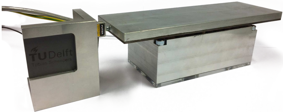
Figure 3.15: Static setup used to measure and verify the generated thrust for different heights
