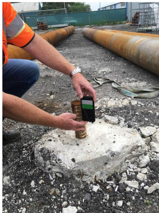
Figure 7.2: Inclination of Pile B1
