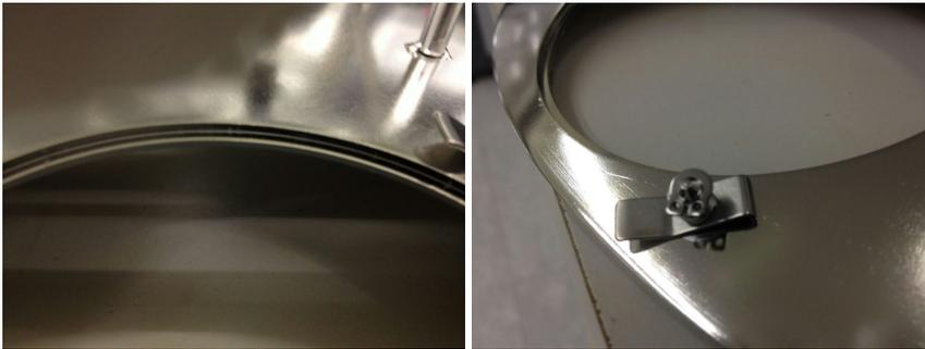
Figure 4.29: The edge of the holder where wafer can be fixed on it and an original clamp of holder.
