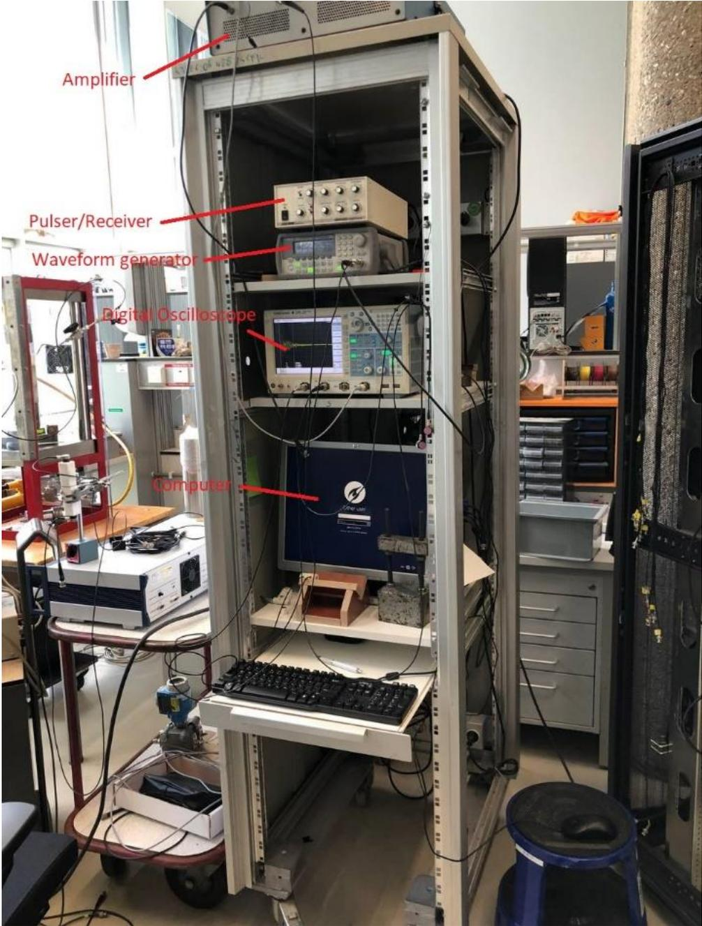
Figure 35: Testing instruments for the UPV test
