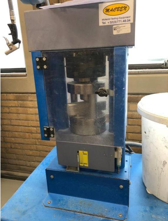
Figure 41: Sample undergoing the 3-point bending test
