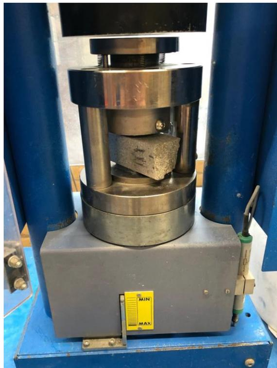
*Figure 43: Sample undergoing the compressive strength test*
