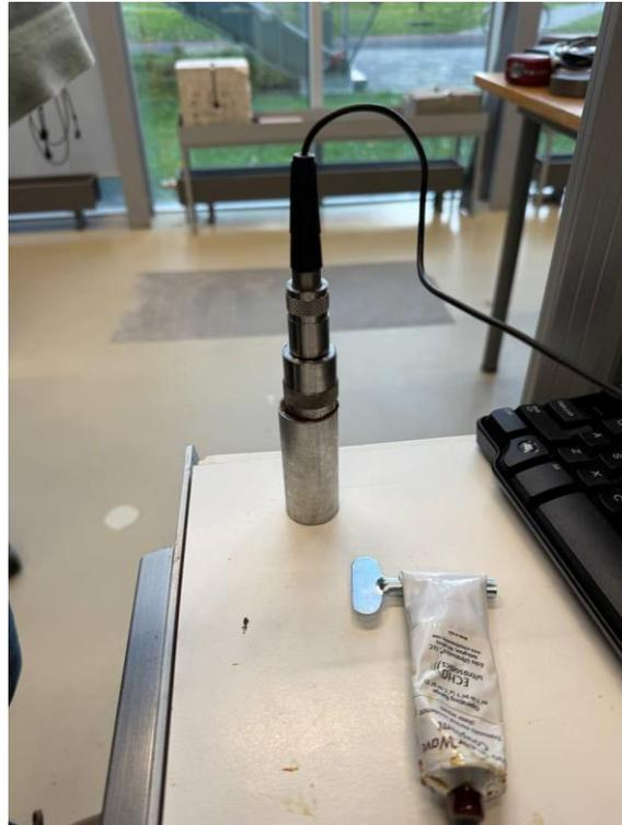
*Figure 36: Calibration of the sensors using the aluminium bar for the Pulse-Echo method*
