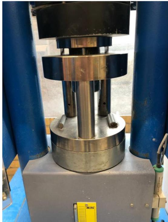
*Figure 40: Setup of the 3-point bending test*
