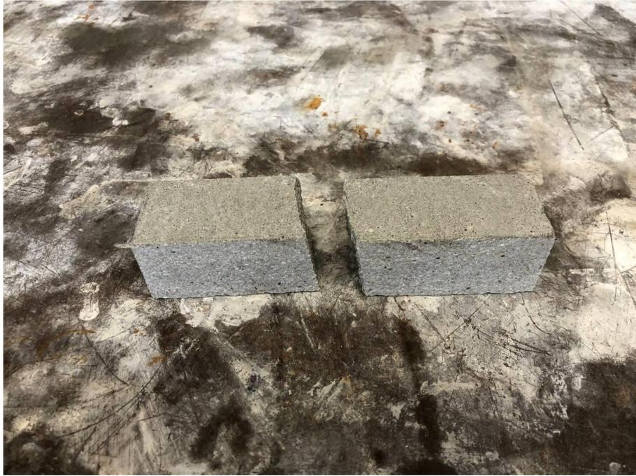
*Figure 42: Sample broken into two pieces after the 3-point bending test*
