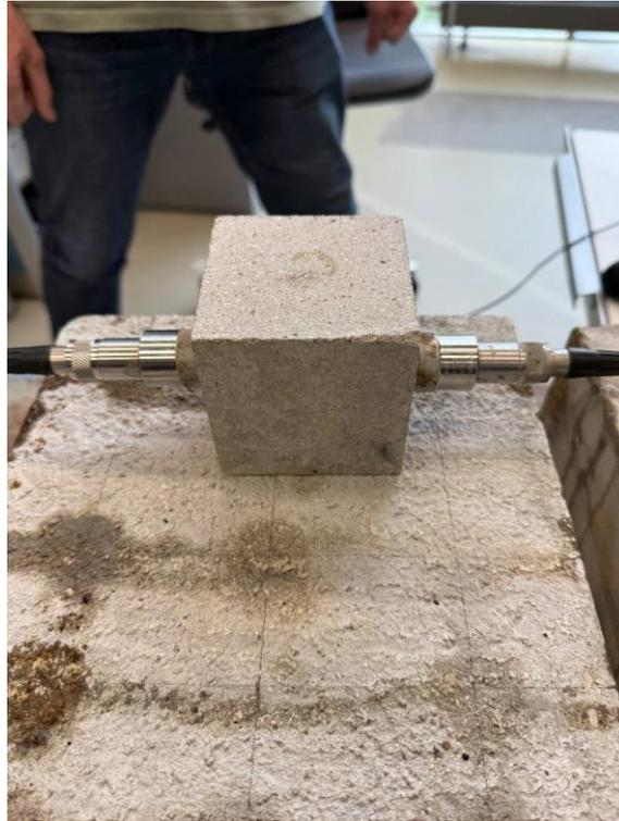
*Figure 48: Setup of the direct transmission method applied to the specimen*
