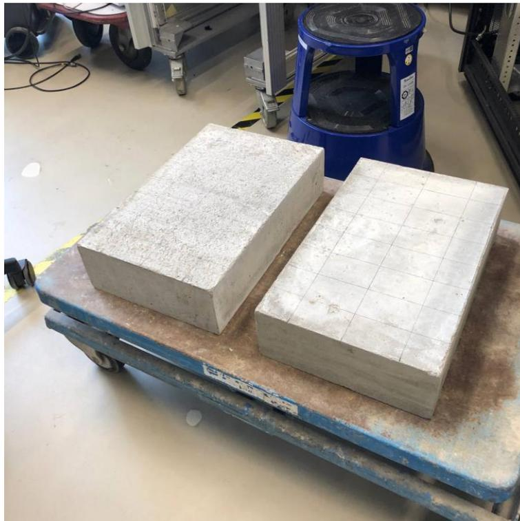
*Figure 34: Marked Samples Indicating Sensor Positions for UPV Testing*
