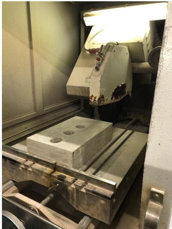
*Figure 38: Concrete samples being cut by a saw*
