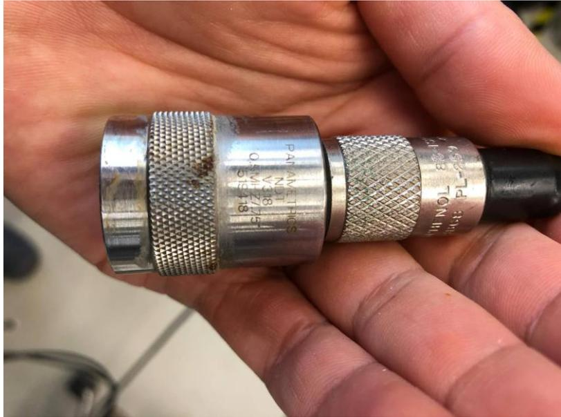
*Figure 37: Transducer used for both the Indirect Methods as the Pulse-Echo Method with a resonant frequency of 500 kHz*
