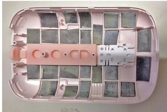
Figure 2.10: Adding weights to a physical model to change acoustics (Timmerman et al., 2022).
