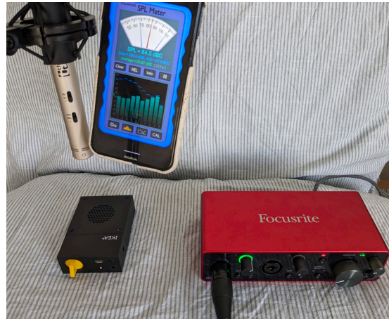
Figure III.III: Setup for Microphone calibration setup.
