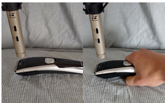
Figure 7.1: Taking separate recordings for the neutral use and with hand force applied.
