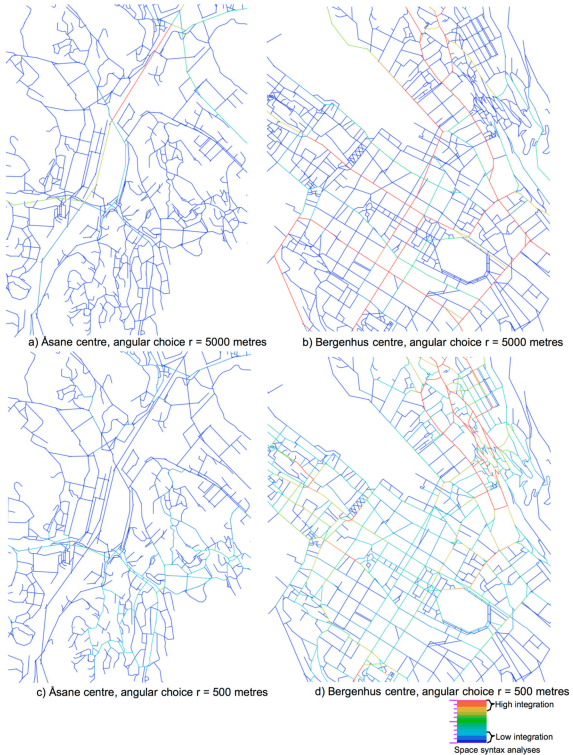
Figure 4. Angular choice analyses of two different centres in Bergen with the two different types of shopping areas with radius like 5000 m (a,b) and radius like 500 m (c,d).
