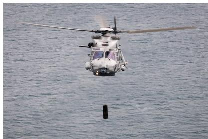
**Figure 3.2:** An NH90 military helicopter in a dipping SONAR mission used by the dutch navy [36]
