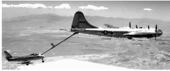
Figure 3.5: United States' Boeing B-29 Superfortress bomber refueling a F-86 with the boom system [8]
