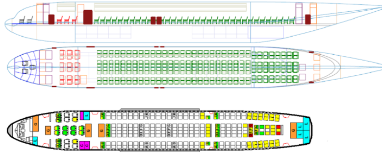
Figure 4.13: Comparison of the KBE fuselage design tool generated fuselage with the fuselage of an A300-600, from Brouwers [12]
