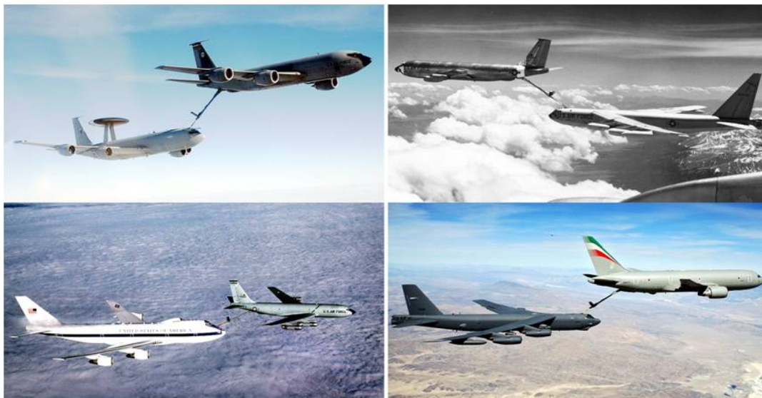
Figure 3.11: In current military in-flight refueling operations, tanker and receiver maintain vertical degree of freedom. Given the typical boom length, it should be noted how close the two airplanes should fly if not in a staggered configuration.
