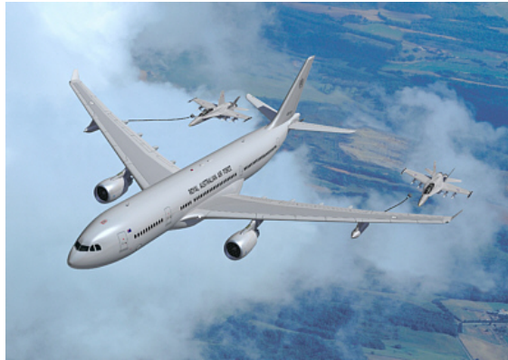
Figure 3.7: Airbus A330 MRTT tanker refueling two F18s at once, from [5]
