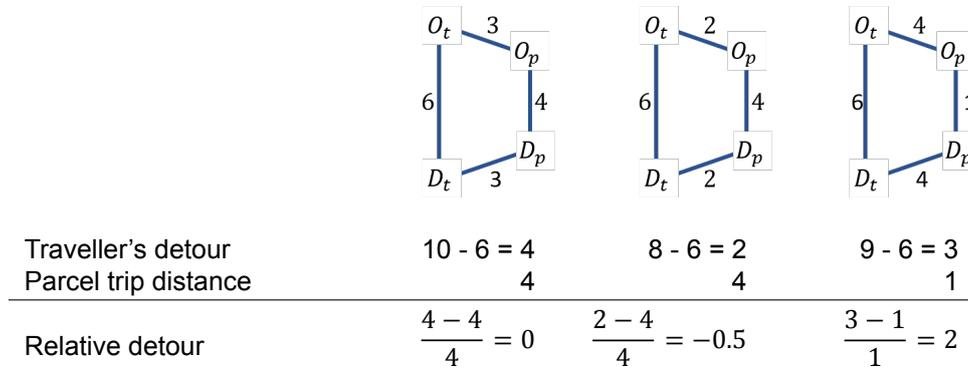
Figure 3.4: Examples relative detour. In each figure clockwise: origin traveller, origin parcel, destination parcel, destination traveller
