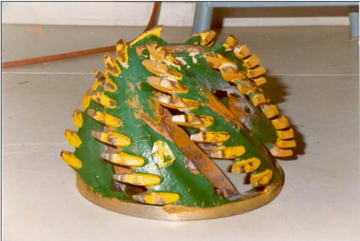
Figure 7-45: The crown cutter head used by Miltenburg (1982).
