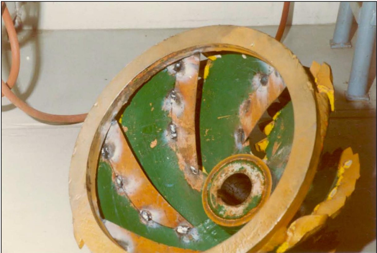
Figure 7-47: Skirts mounted inside the crown cutter head.
