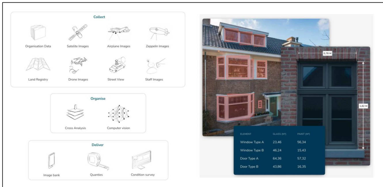
Figure 96: Overview of the condition assessment process of facades using emerging technology. Source: facadeserviceapplicatie.nl
