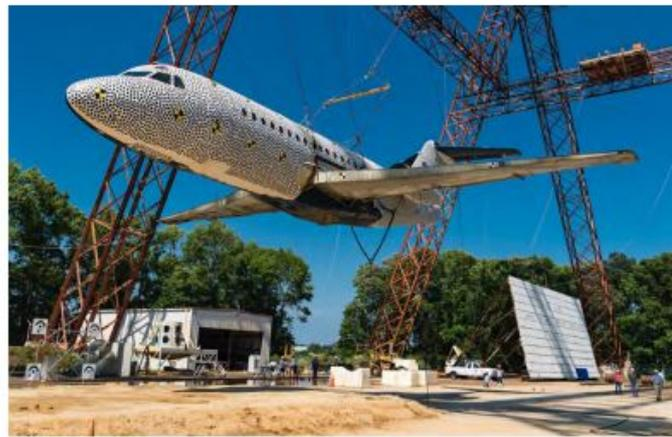
(b) The full F28 structure used for the drop test, which was slightly modified and painted with black dots for collecting photogrammetric data.
