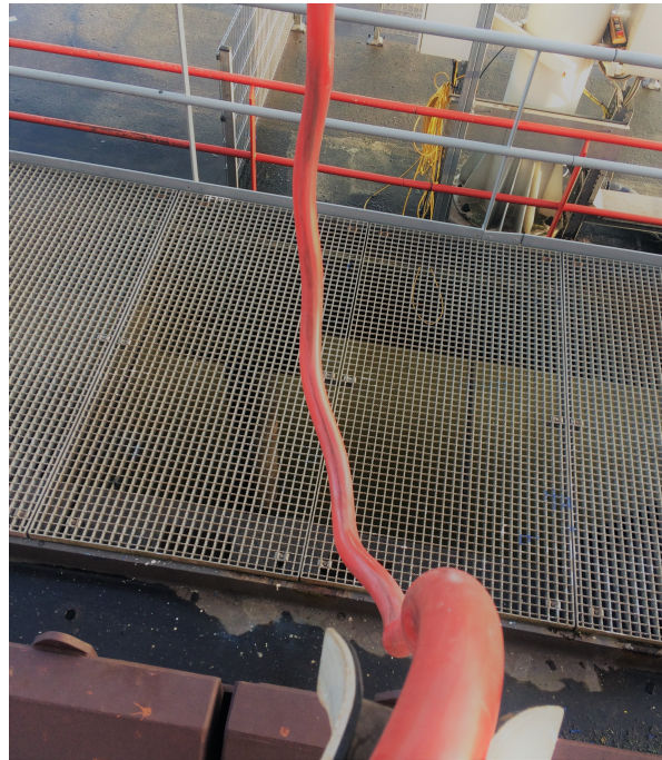
Figure 3.31: The power cable of the charging mechanism of the Stena Line which is plastic deformed.
