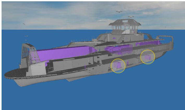
Figure 3.17: The location of the batteries in the current design of the vessel for BC Ferries.
