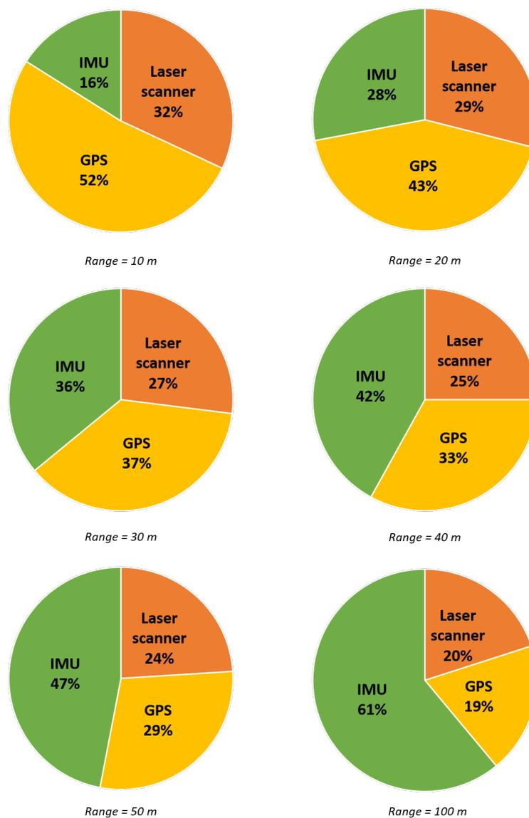
Figure 5.8: Percentage contribution of each one of the three components (laser scanner, GPS and IMU) to the positioning accuracy for different values of the range, 10 m, 20 m, 30 m, 40 m, 50 m and 100 m.
