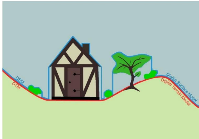
Figure 6.3: The difference between a Digital Surface Model (DSM) and a Digital Terrain Model (DTM). Source: [45]
