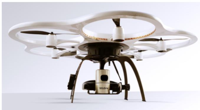
Figure 3.1: The Aibot X6 hexacopter, manufactured by Aibotix, with the Velodyne HDL-32E laser scanner on board. A characteristic example of an aerial system for UAV Laser Scanning. Source:[28]
