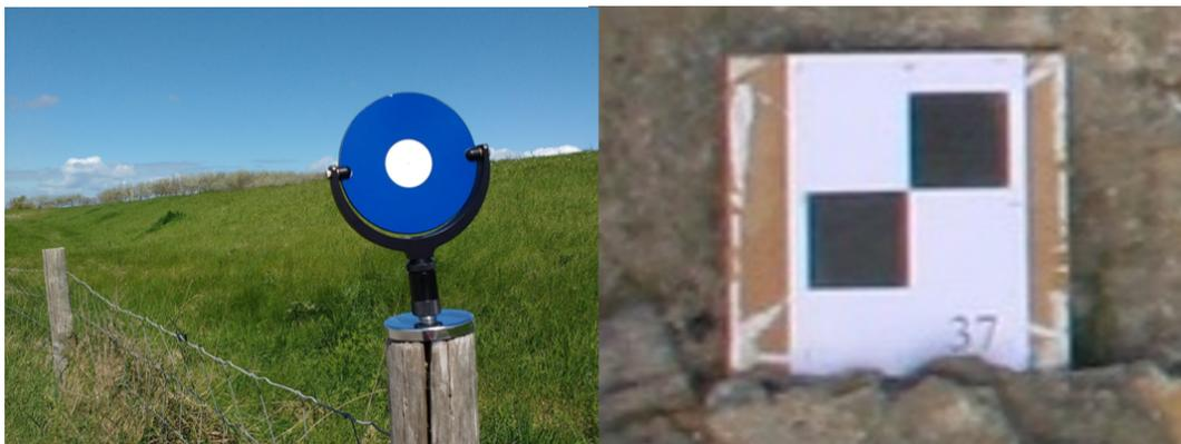
Figure 4.5: Left: Leica round target. Right: Square target
