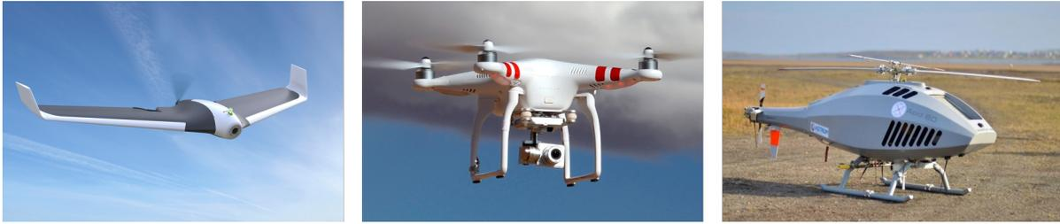
Figure 3.4: Left: Fixed-wing drone. Middle and right: Rotary-wing drones (quadcopter and helicopter). Source: [35], [12], [16]
