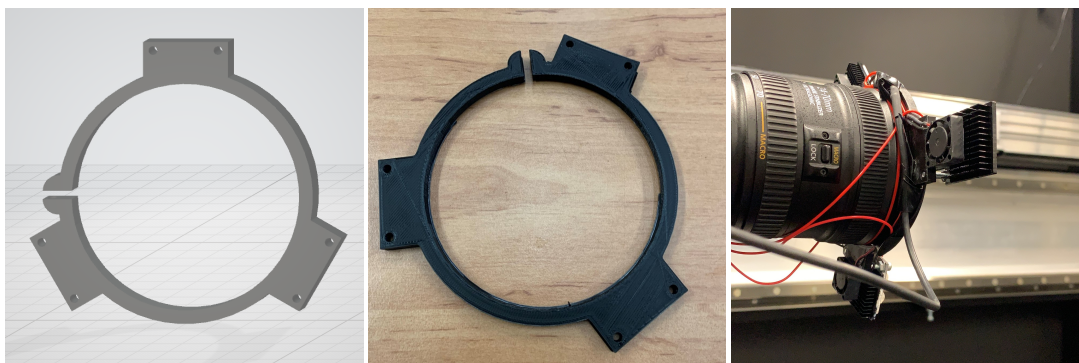
Figure 7.2: Led mount. From left to right, drawing of mount, printed mount, integrated mount with active cooling.
