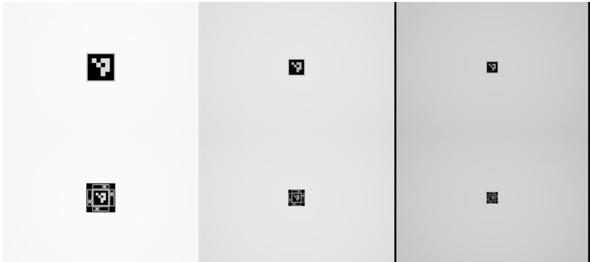
Figure 8.1: Sample of test images at ranges of 1.3, 2.3 and 3.3 metres.
