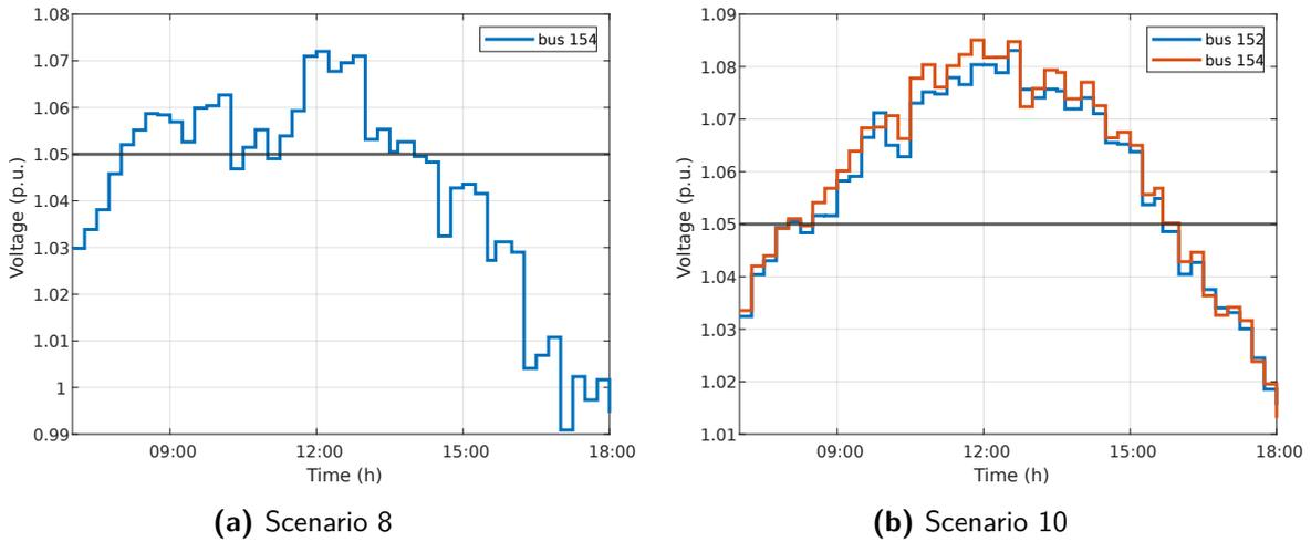
**Figure 5-6:** Two scenarios of the tuning dataset that indicate when the first voltage violation occurs, when there is no curtailment. The time-instance of the first overvoltage violation determines the starting time of the curtailment. In scenario 8, the first overvoltage occurs at 8:00 a.m. in bus 154 and in Scenario 10 the first overvoltages occur at 8:00 a.m. in bus 152 and bus 154.
