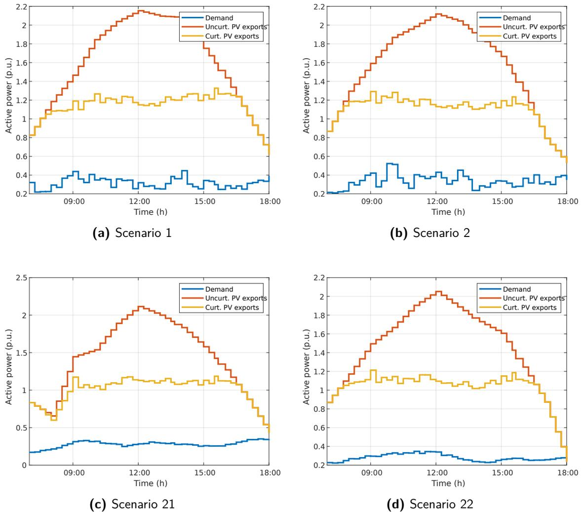
**Figure 5-9:** Residential demand compared to uncurtailed PV exports and curtailed PV exports after DRCCP with  $\theta = 10^{-4}$  for 4 scenarios. The low residential demand without high fluctuations determines the shape of the curtailed PV exports.
