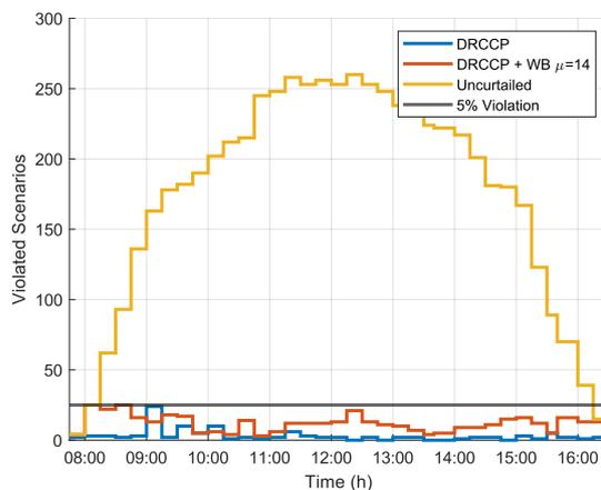
(b) Number of scenarios with overvoltage violations without curtailment and with curtailment for the DRCCP approach with 20 tuning scenarios with the DRCCP approach with the Wasserstein Barycenters. The violated scenarios dominate when there is no PV control.
