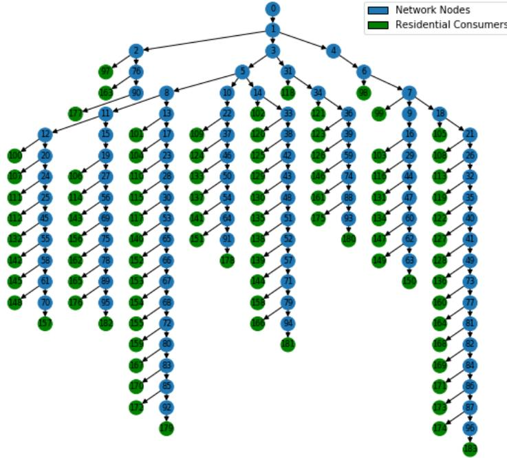
**Figure 5-1:** The network to implement the DRCCP algorithm. This network is part of the Dutch network and consists of 1 slack bus, 96 connecting buses with no demand and PV generation and 87 residential buses with PV installations.
