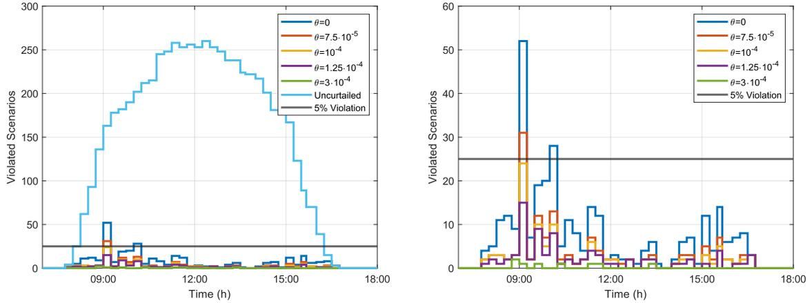
(a) Number of scenarios with overvoltage violations without curtailment and with curtailment for different values of  $\theta$ . (b) Number of scenarios with overvoltage violations after curtailment for different values of  $\theta$ .
