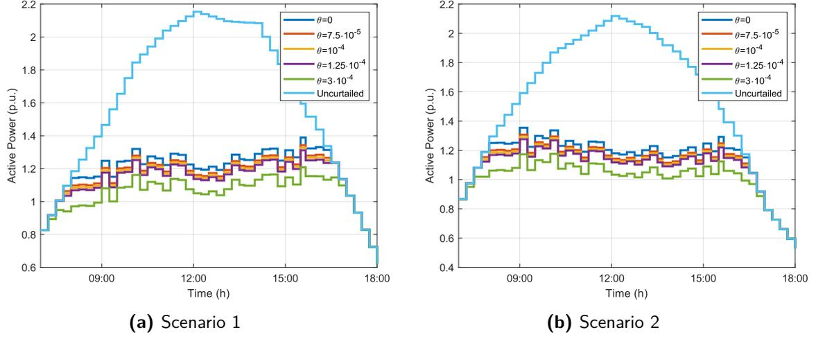
**Figure 5-5:** Uncurtailed PV contribution compared to PV contribution under curtailment with different Wasserstein radii  $\theta$  for two scenarios. The available PV exports after curtailment do not present any high peaks during the whole day and they decrease monotonically as we increase the Wasserstein radius  $\theta$ .
