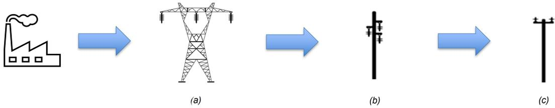
**Figure 4-1:** The energy grid (a) Transmission, (b) Subtransmission, (c) Distribution networks [29].
