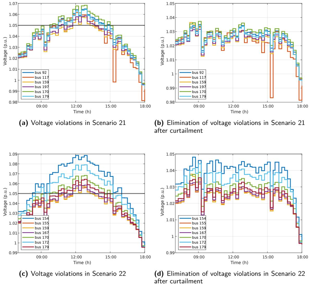
**Figure 5-8:** Voltage magnitudes before and after curtailment in two unseen scenarios. On the left side, the voltage magnitudes of 6 buses in Scenario 21 and 7 buses of Scenario 22 that present overvoltage issues, when we do not implement PV curtailment. On the right side, the same buses of Scenario 21 and Scenario 22 when we run the DRCCP algorithm with  $\theta = 10^{-4}$ . After implementing curtailment, the voltage magnitudes of the buses lie below the limitation of 1.05 p.u.
