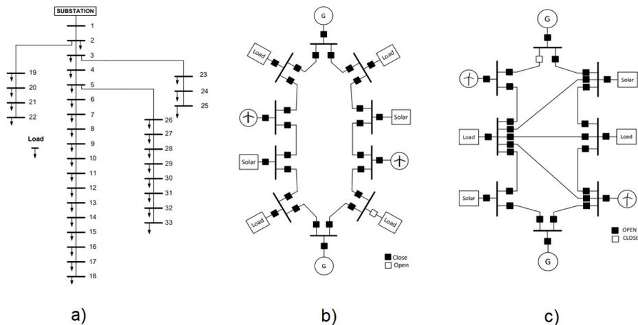
**Figure 4-2:** Types of Distribution Systems (a) Radial, (b) Loop, (c) Meshed. The radial topology is the most economical type of distribution networks and it has a tree shape. The loop topology is more expensive, but it is more reliable and the meshed topology consists of multiple loop topologies [31].
