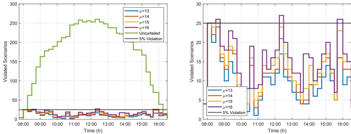
**(a)** Number of scenarios with overvoltage violations without curtailment and with curtailment for different values of  $\mu$  and  $\theta = 10^{-4}$  **(b)** Number of scenarios with overvoltage violations after curtailment for different values of  $\mu$  and  $\theta = 10^{-4}$
