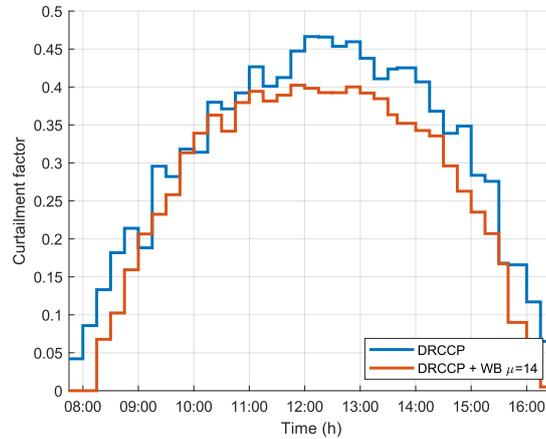
(a) Comparison of curtailment factors at every time instance of the DRCCP approach with 20 tuning scenarios with the DRCCP approach with the Wasserstein Barycenters. The curtailment factors of the DRCCP approach with the Wasserstein Barycenters are mainly smaller than the DRCCP approach with 20 tuning scenarios.
