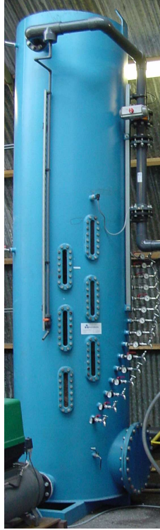
Figure 2.10: Photograph of the multimedia filter, which is used in the pilot investigations
