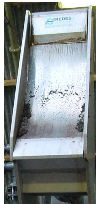
Figure 2.9: Photograph of the curved sieve, which is used in the pilot investigations
