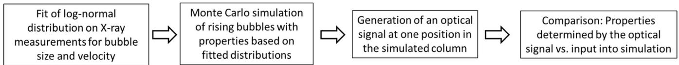
Fig. 22. Schematic procedure of the Monte Carlo simulation.
