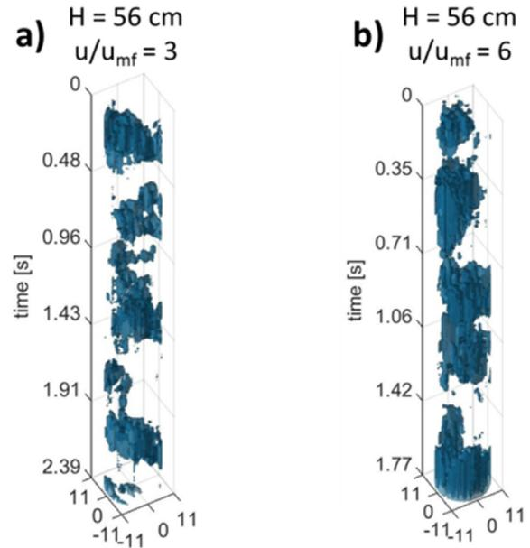
Fig. 21. Reconstructed bubbles at H=56cm for fluidization numbers of 3 and 6 based on X-ray measurements.
