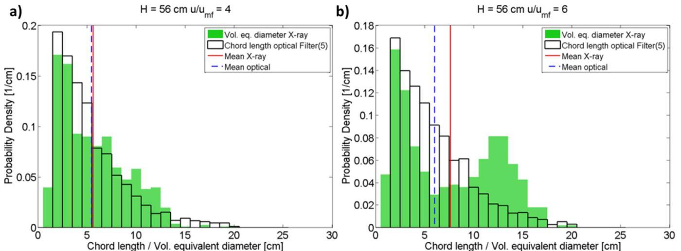
Fig. 20. Histograms of the chord length distribution for the filtered artificial optical signal and the volume equivalent diameter (above the entire cross-section) for the X-ray evaluation at H = 56 cm and  $u/u_{mf}$  = 4 and 6.
