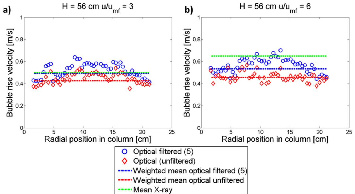
**Fig. 14.** Mean BRV from X-ray evaluation (solid line) and mean annulus weighted BRV from optical evaluation (dashed lines). Each radial measurement point matches with the mean BRV of the corresponding pixel on the evaluation path in Fig. 3(c). (For interpretation of the references to color in this figure legend, the reader is referred to the web version of this article.)
