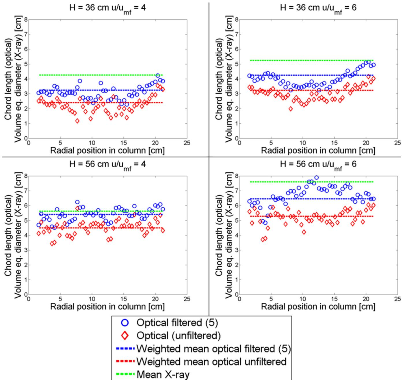
**Fig. 18.** Mean bubble size from X-ray evaluation (green dashed line) and mean annulus weighted chord lengths from optical evaluation (red and blue dashed lines). Each radial measurement point matches with the mean chord length of the corresponding pixel on the evaluation path in Fig. 3(c). (For interpretation of the references to color in this figure legend, the reader is referred to the web version of this article.)
