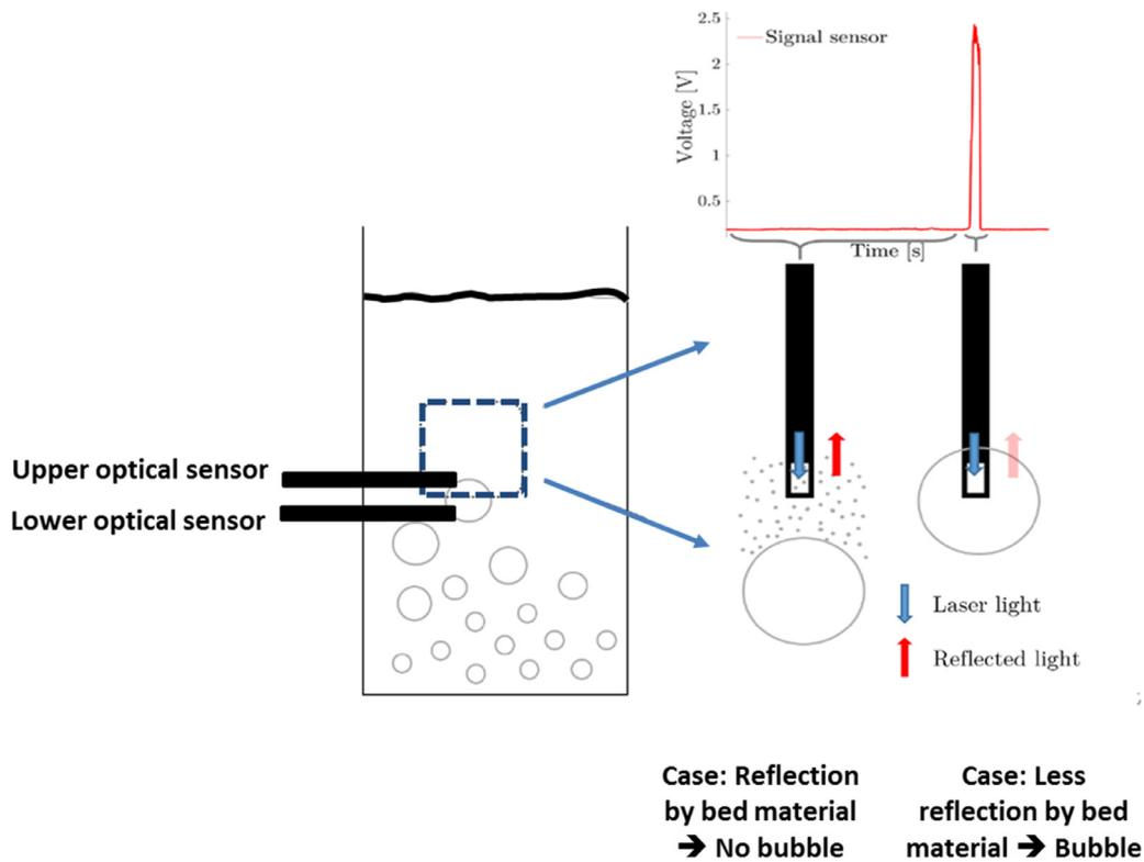
Fig. 1. Measurement principle of the optical sensor.
