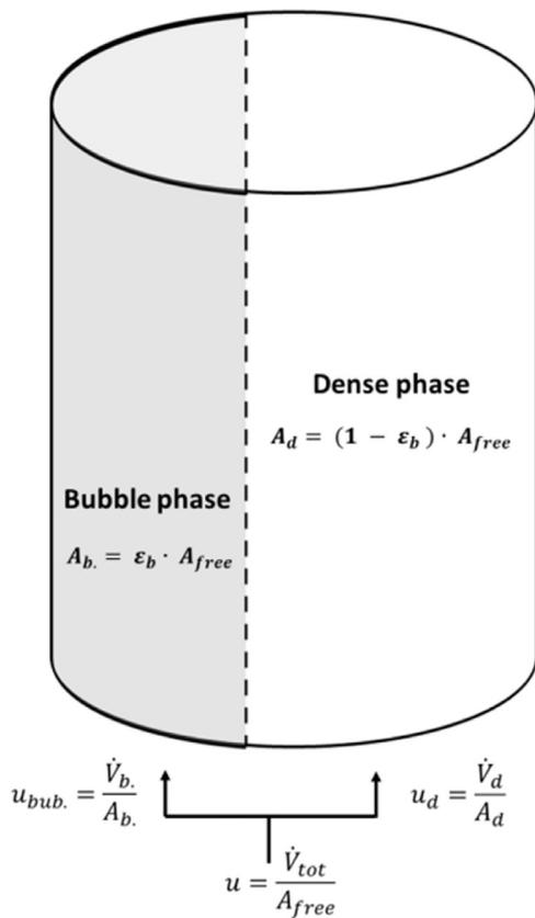
Fig. 2. Schematic view on the classical two-phase model.
