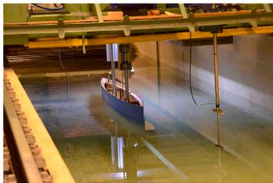
Fig. 16. The wigley hull model in the towing tank.
