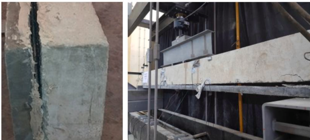
Fig. 24. Debonding at the interface [52,107].
