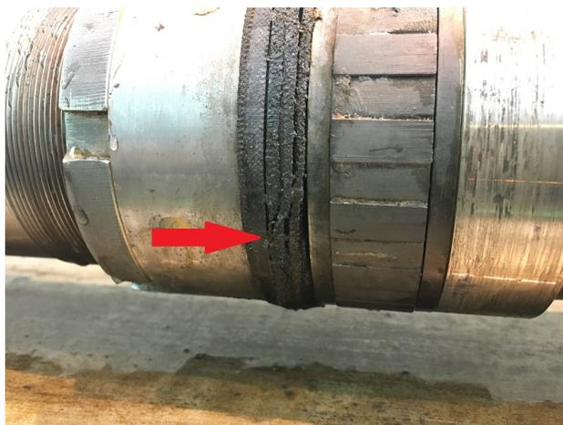
Figure 5.24: Tearing of glued connection due to pressure
