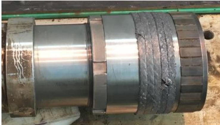
Figure 4.8: Installation of packing rings on housing
