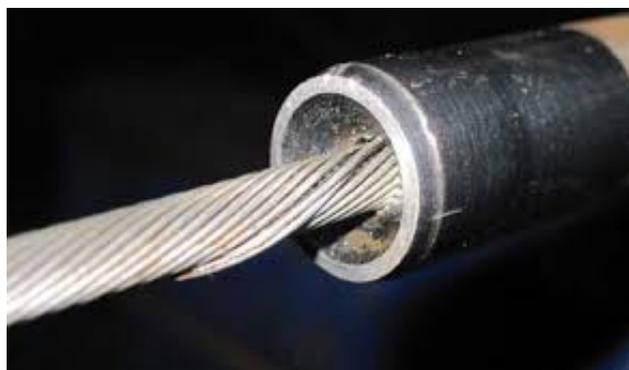
Figure A.13: Example of uneven surface for wireline braided cable
