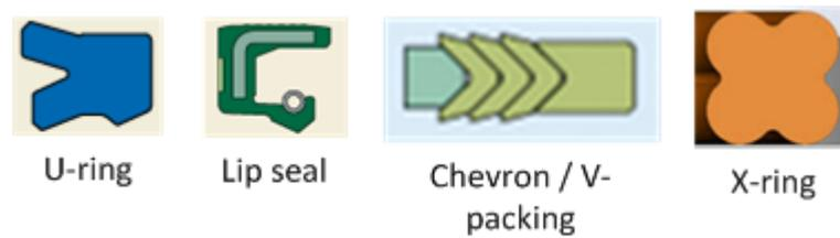
Figure A.3: Different types of cross-sectional shapes
