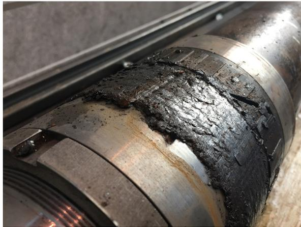
Figure 5.18: Deformation of packing seal due to moving of SOCCS casing
