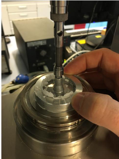
Figure 5.6: Prevention of extrusion of fluid during measurement
