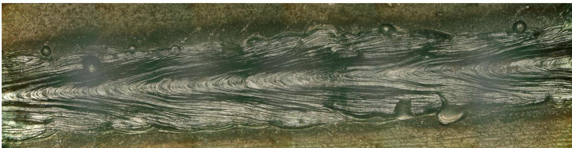
Figure 3.2: Light microscope image of weld
