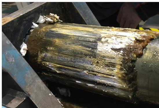
Figure 5.10: Results of bleeding of polymers out of rubber
