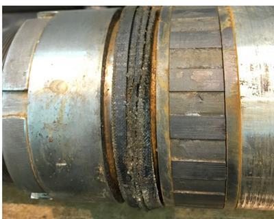
Figure 5.25: Twisting of chevron set due to contact with bottom of SOCCS casing
