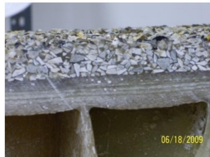
(b) Interface flange with polymer concrete
