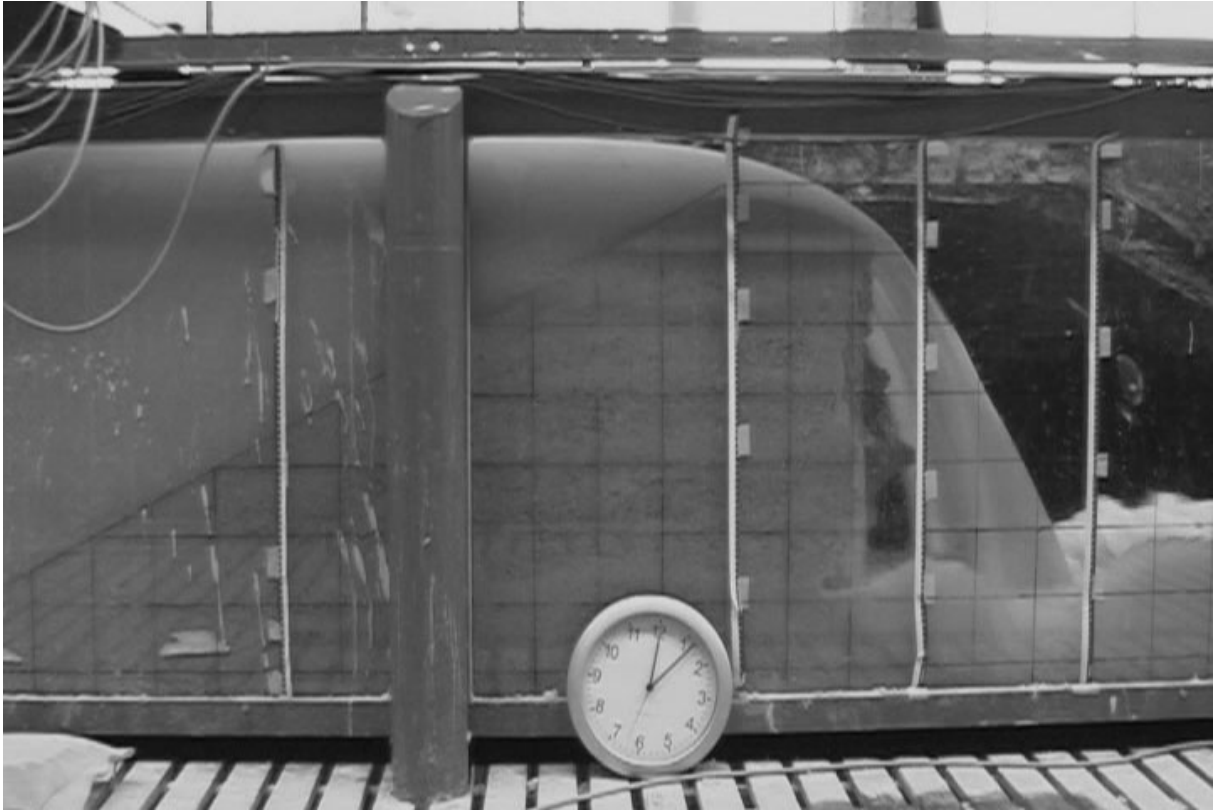
Figure 6.13 Headcut and breach flow jet impingement (test T 4 ).
