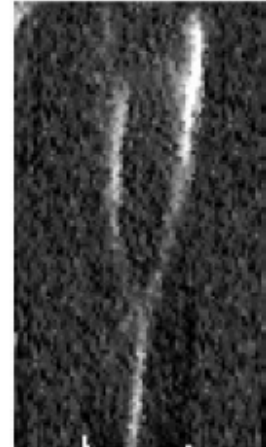
Figure 2-4: Two particles ( \sim 8\mu\text{m} ) entrained in a horizontal acoustic field and vertical gravity, the particles have the same size and have an initial particle separation of around 140\text{-}150\mu\text{m} and collide within 20ms at 5kHz, V=0.44\text{ m/s} , Re=0.23 [1]
