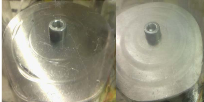
Figure 5-9: Ring shaped deposition on the radiation plate while the transducer was turned off (left) and on (right). The shape of the radiation plate appears to be deform due to the optical properties of the agglomeration chamber.
