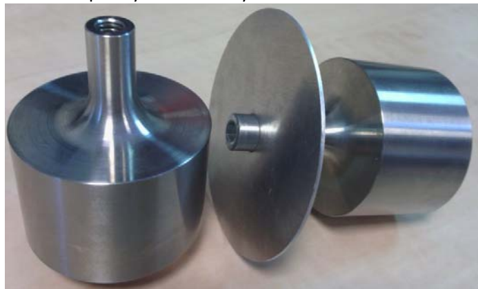
Figure 3-3: Two ultrasonic horns, one with a flexure mode radiation plate.
