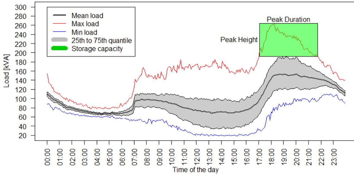
Figure 2: Design of storage unit for neighbourhood 1 (100% residential connections)
