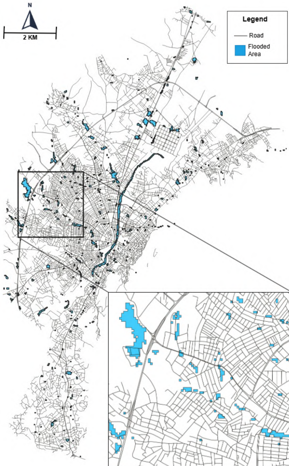
Figure 4.5: Q100 Arc-Malström flood model output of Antakya as visualized in QGIS. Flood depths > 0.5 m are shown in blue.
