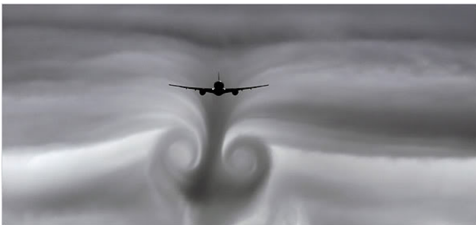
Figure 3.2: Wake turbulence as it was captured in this picture when a British Airways flight was descending through thin clouds near London in July 2006 [Stellin, 2007].
