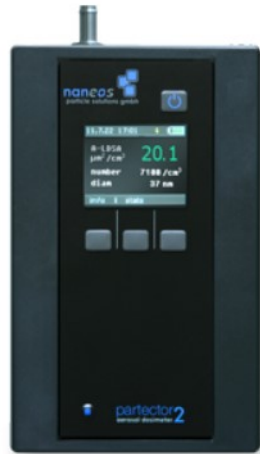
Figure 2.2: The Naneos partector used for measuring particulate matter [43]
