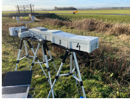
Figure 2.3: The 4 gas sensor boxes positioned next to the Polderbaan at Schiphol used for measuring gaseous pollutant
