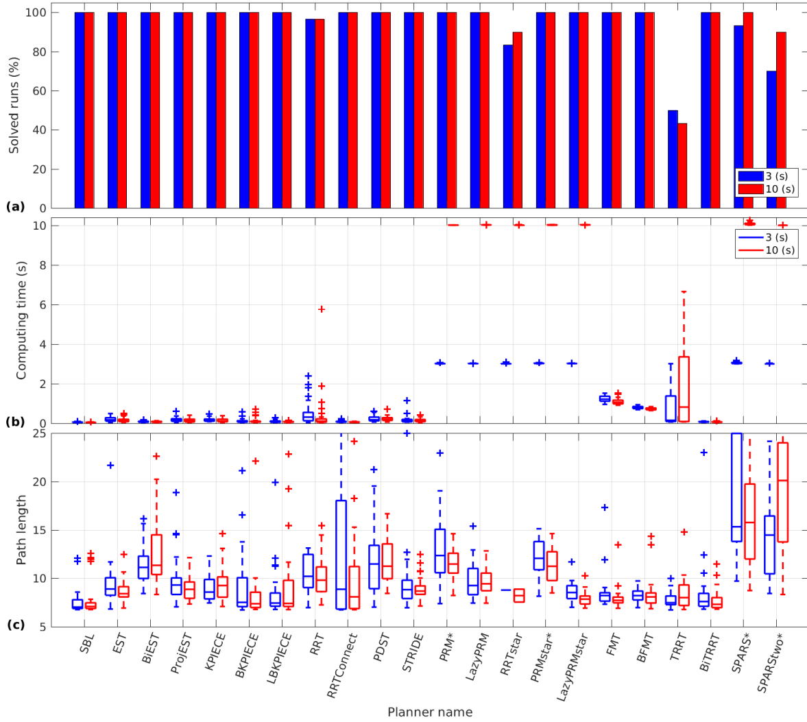
Fig. 5: Results for benchmark 2 for 3s and 10s maximum computing time. a. Solved runs (higher is better), b. Computing time (lower is better, small interquartile range is better), c. Path length (lower is better, small interquartile range is better).
