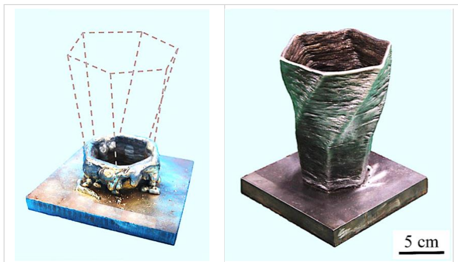
Figure 5: Thin wall twist bottle produced by the wire and arc additive manufacturing process. [a] Natural cooling; [b] Active substrate cooling [13].
