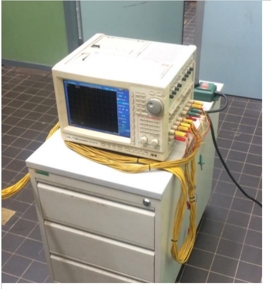
Figure 18: The experimental measurement values are acquired by a digital scope; Yokogawa DL716 [28].
