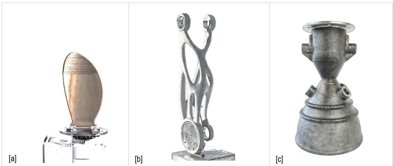
Figure 2: Components that are produced by the wire and arc additive manufacturing process. [a] Hollow propeller blade, NiBrAl; [b] Robot arm with optimized topology, stainless steel 316L; [c] Rocket Thruster with added functionalities, stainless steel 308L [6].
