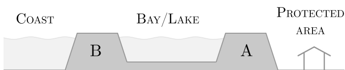
Figure 1: Simplified cross section of a front defense (B) and rear defense (A).
