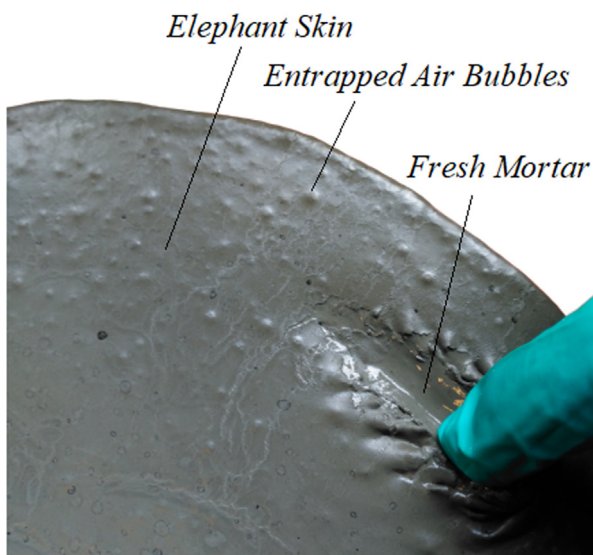
Fig. 3. Elephant skin formation just after slump-flow.
